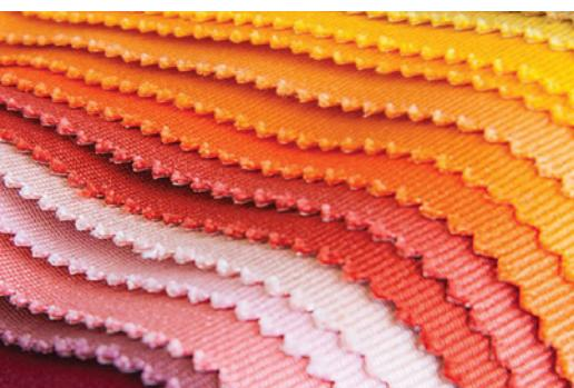
Repreve® SmartDye : this recycled polyester can be dyed at a lower temperature than standard polyester, yielding substantial energy savings and reducing dyeing-cycle time. Many yarns may be dyed at atmospheric pressure, lower-temperature dyeable recycled polyester improves the efficiency of the dyeing cycles and achieves up to 30% energy savings without compromising your fabric's performance.
